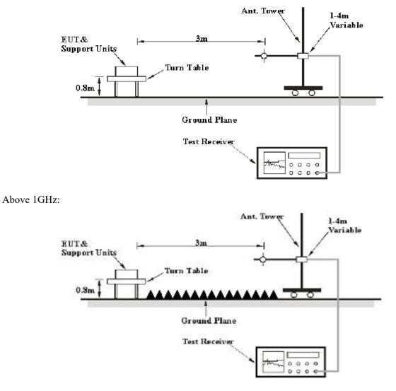
The radiated emission were performed in the 3 meters chamber test site, using the setup accordance with the ANSI C63.4-2014. The specification used was with the FCC Part 15 B Class B limits.
