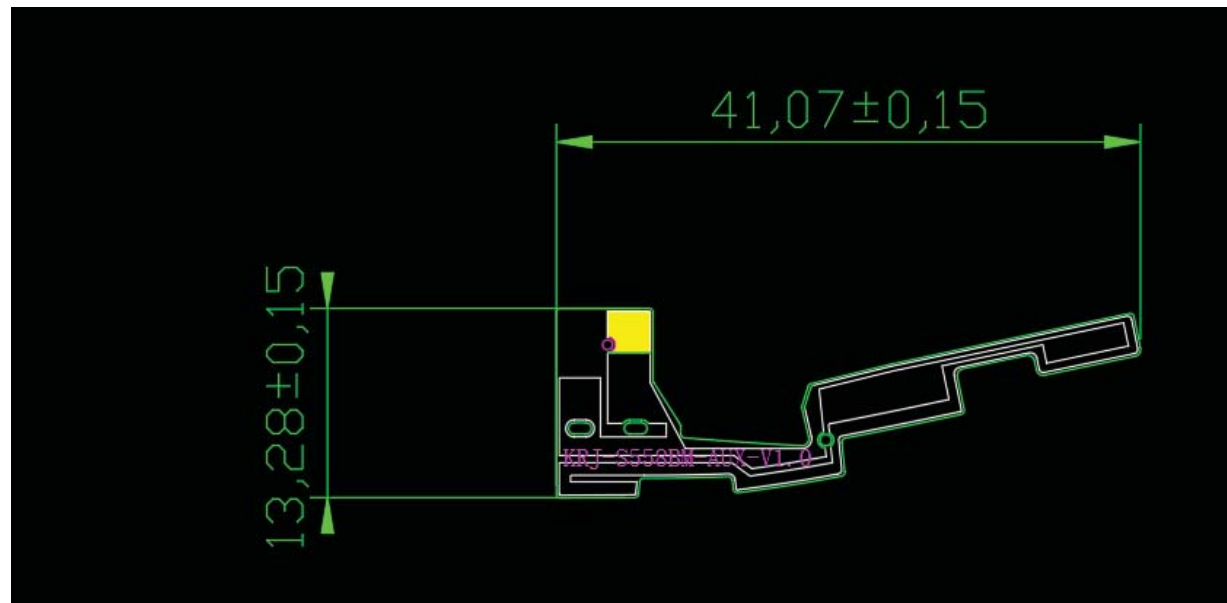
Dimensional diagram of diversity antenna
