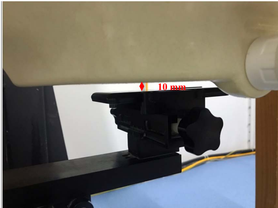
Body (Worn) Back Setup Photo (10mm)
