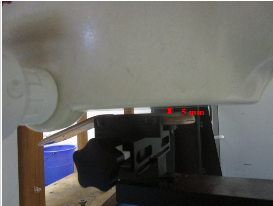
Body Worn Back Setup Photo (5mm)
