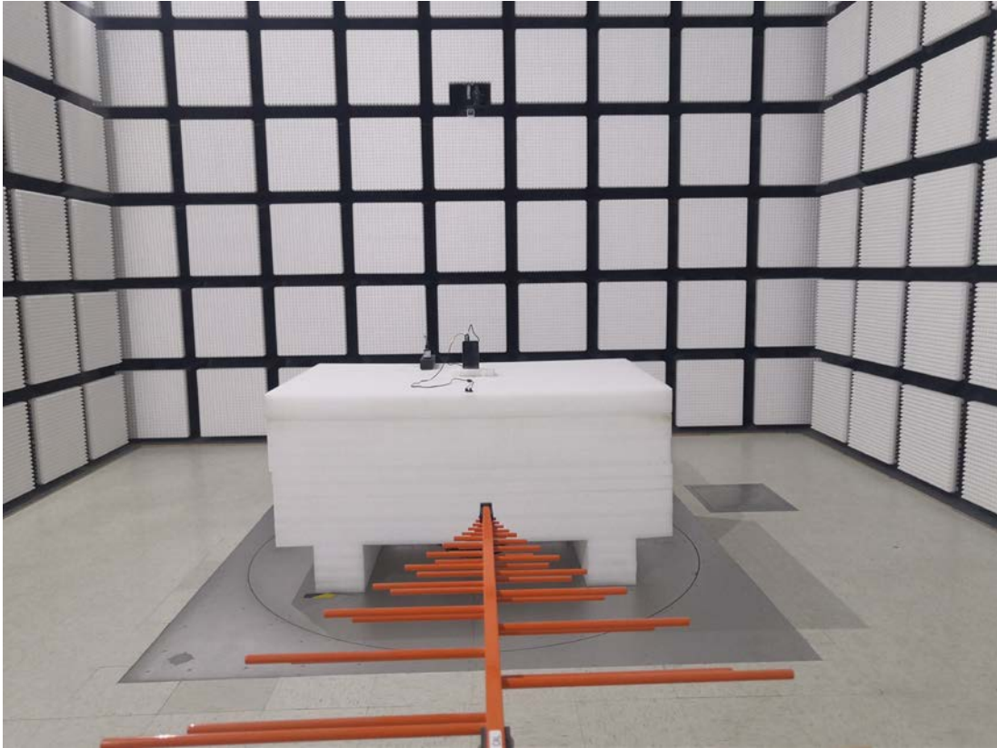
Radiated Emission Below 1GHz View -Adapter 2#
