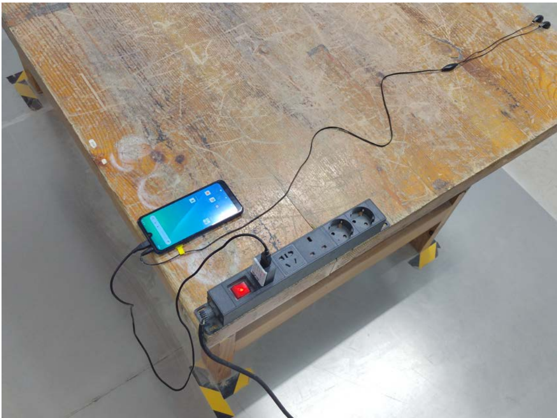
Conducted Emissions Side View -Adapter 2#
