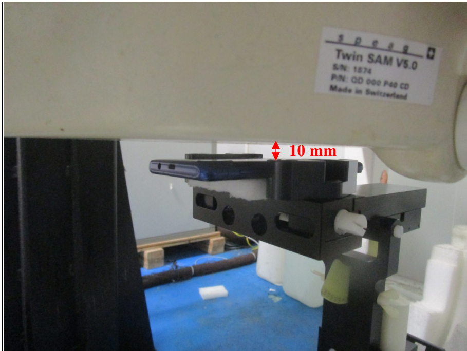
Body (Worn) Front Setup Photo (10mm)
