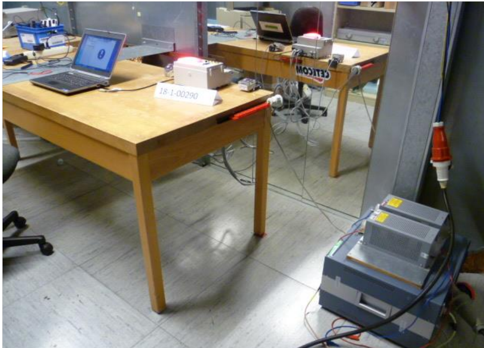
Photograph 5: EUT Setup Conducted emissions on AC-Power lines
