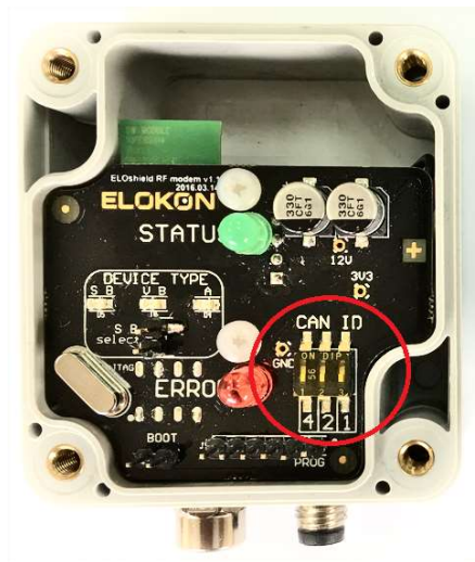
Figure 9. The vehicle antenna module (A) with the cover removed and the switch marked in red provided to set the CAN ID address
