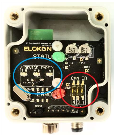
Figure 16. Antenna module (A) with the cover removed, the switch marked in red provided to set the CAN ID address and the SB select jumper marked in blue.
