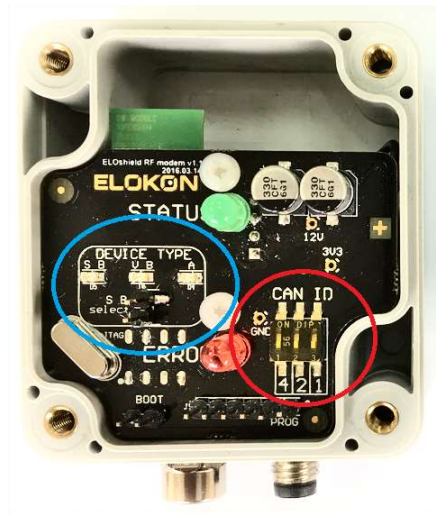
Figure 17. Stationary antenna module (B) with the cover taken off. Marked in red is the switch used to set the CAN ID address. Also marked, in blue, is the link used to set its operation mode as a vehicle antenna module (B) or stationary antenna module (B).
