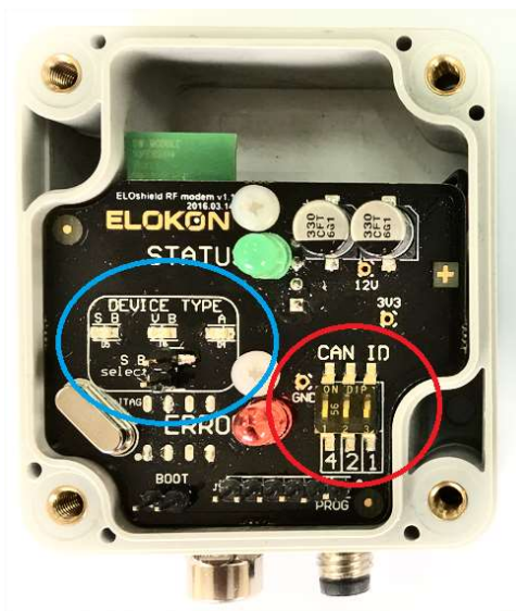
Figure 10. The antenna module (B) with the cover removed and the switch marked in red provided to set the CAN ID address. Blue circle shows the jumper used to set the operating mode as the vehicle antenna module (B) or as the stationary antenna module (B).
