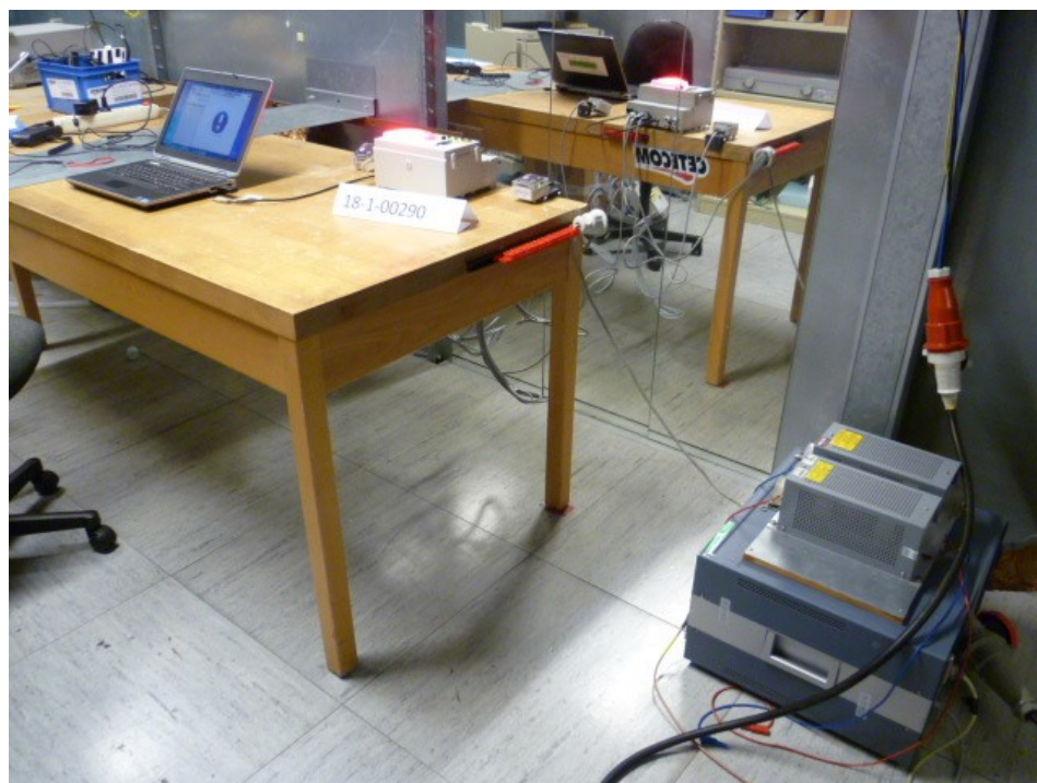
Figure 2: EUT A Verification Module conducted AC emission set up
