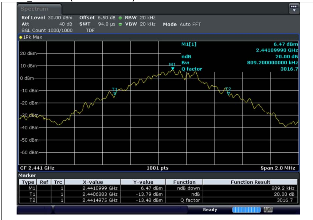
GFSK 2 441 MHz(20 dB Bandwidth)
