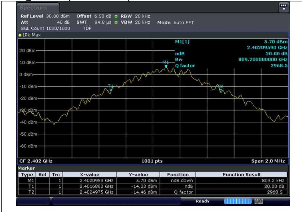
GFSK 2 402 MHz(20 dB Bandwidth)
