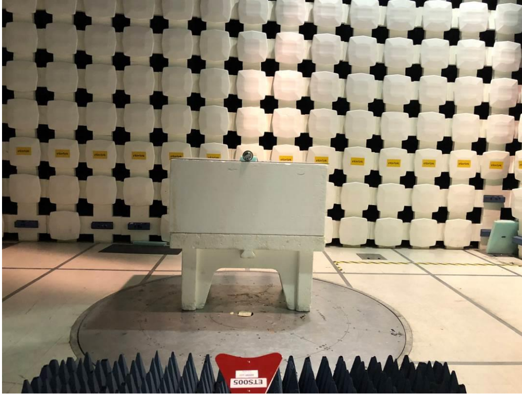
Radiated Emissions Test Setup, Above 1000 MHz
