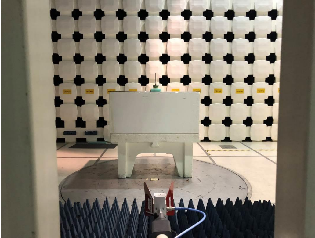
Radiated Emissions Test Setup, Above 1000 MHz
