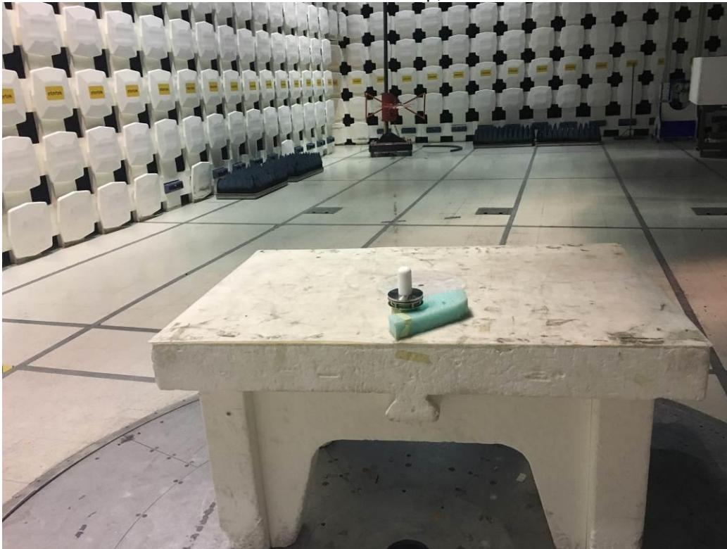
Radiated Emissions Test Setup, 30-1000 MHz
