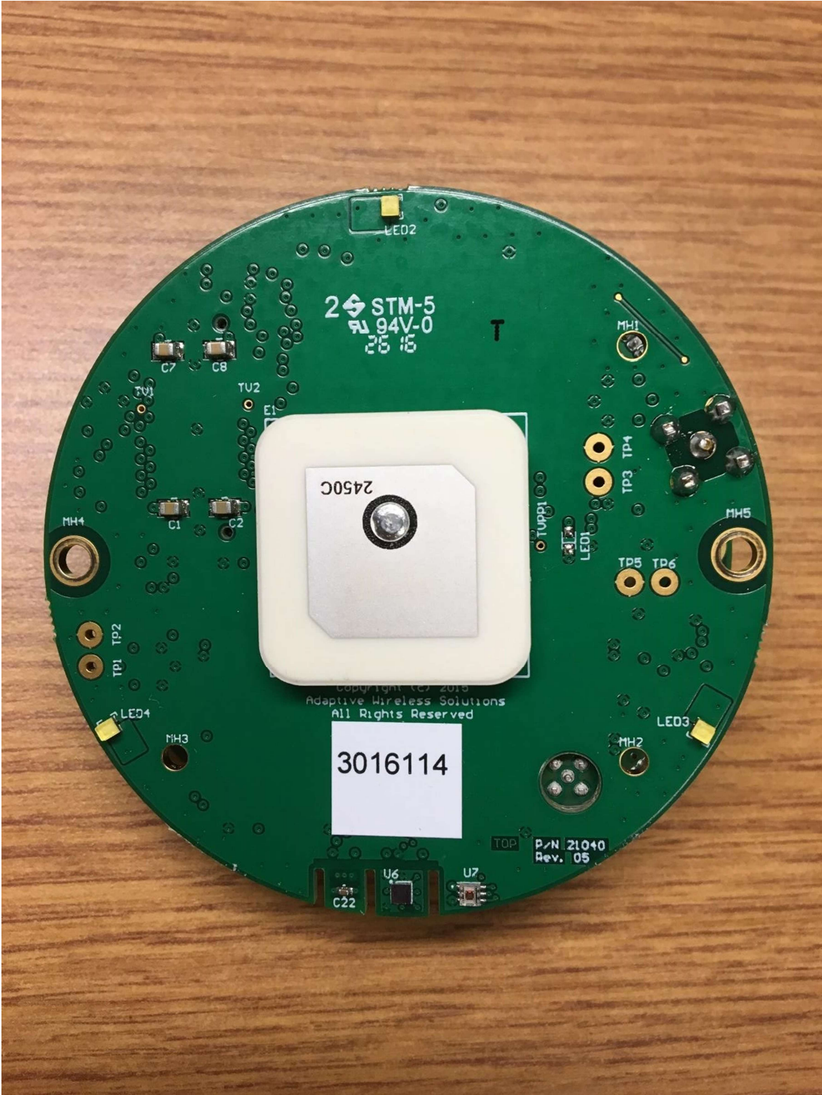
Top of RF PCB (BLE WLP.2450.25.4.A.02 antenna)
