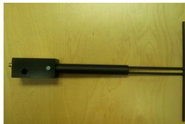
Figure 1 – MVG COMOSAR Validation Dipole
