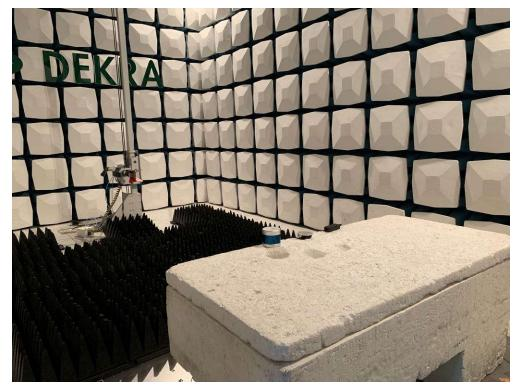
Test Mode: Mode 1-4 Description: Rear View of Radiated disturbance Test Setup (Above 1GHz)
