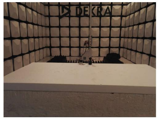
Test Mode: Mode 1: Full System Description: Rear View of Radiated Disturbance Test Setup (Above 1GHz)
