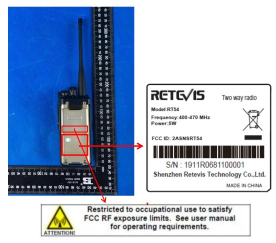
The label shown shall be permanently affixed at a conspicuous location on the device and be readily visible to the user at the time purchase (Labeling requirement per 2.925)
