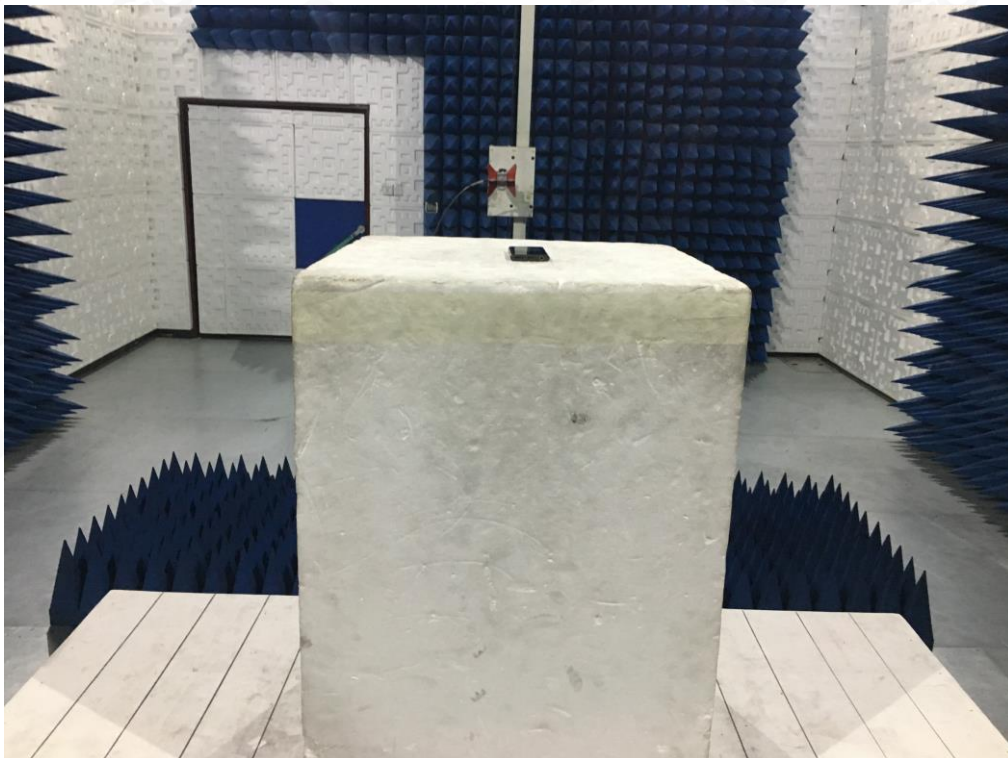
RADIATED EMISSION TEST SETUP ABOVE 1GHZ
