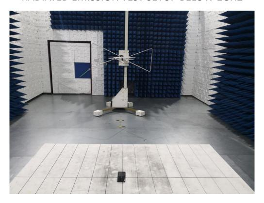
RADIATED EMISSION TEST SETUP ABOVE 1GHZ
