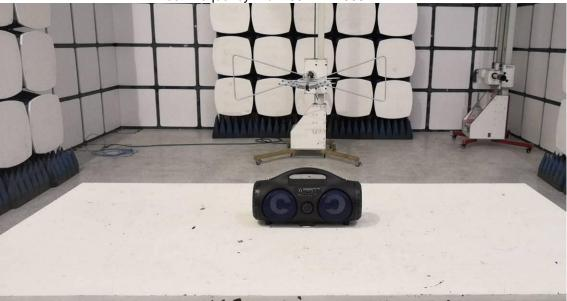
Test Frequency From 1000MHz-26.5GHz
