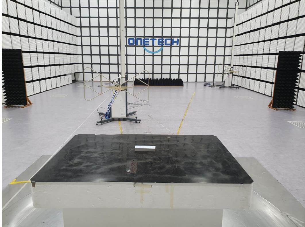
**- Radiated Emission Test (Above 1 GHz)**
