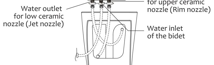
**3** Connect the bidet hose to the water inlet of the bidet.
