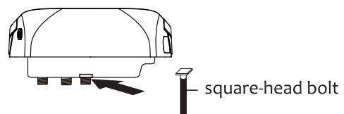
**4** Insert a square-head bolt to the groove at the bottom of the bidet.
