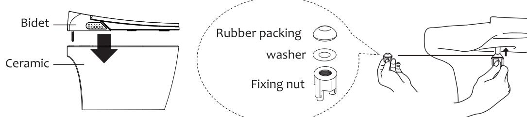
**5** Insert the square-head bolt into an installation hole on the ceramic fix the bolt with rubber packing, washer and nut.
