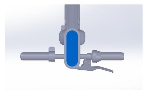
In addition, the Module must only be mounted to a stem that shares the same stem and handlebar geometry as the SCT-03-0-x in order to ensure that the NFC antenna is isolated from the metal in the scooter handlebar and stem.
