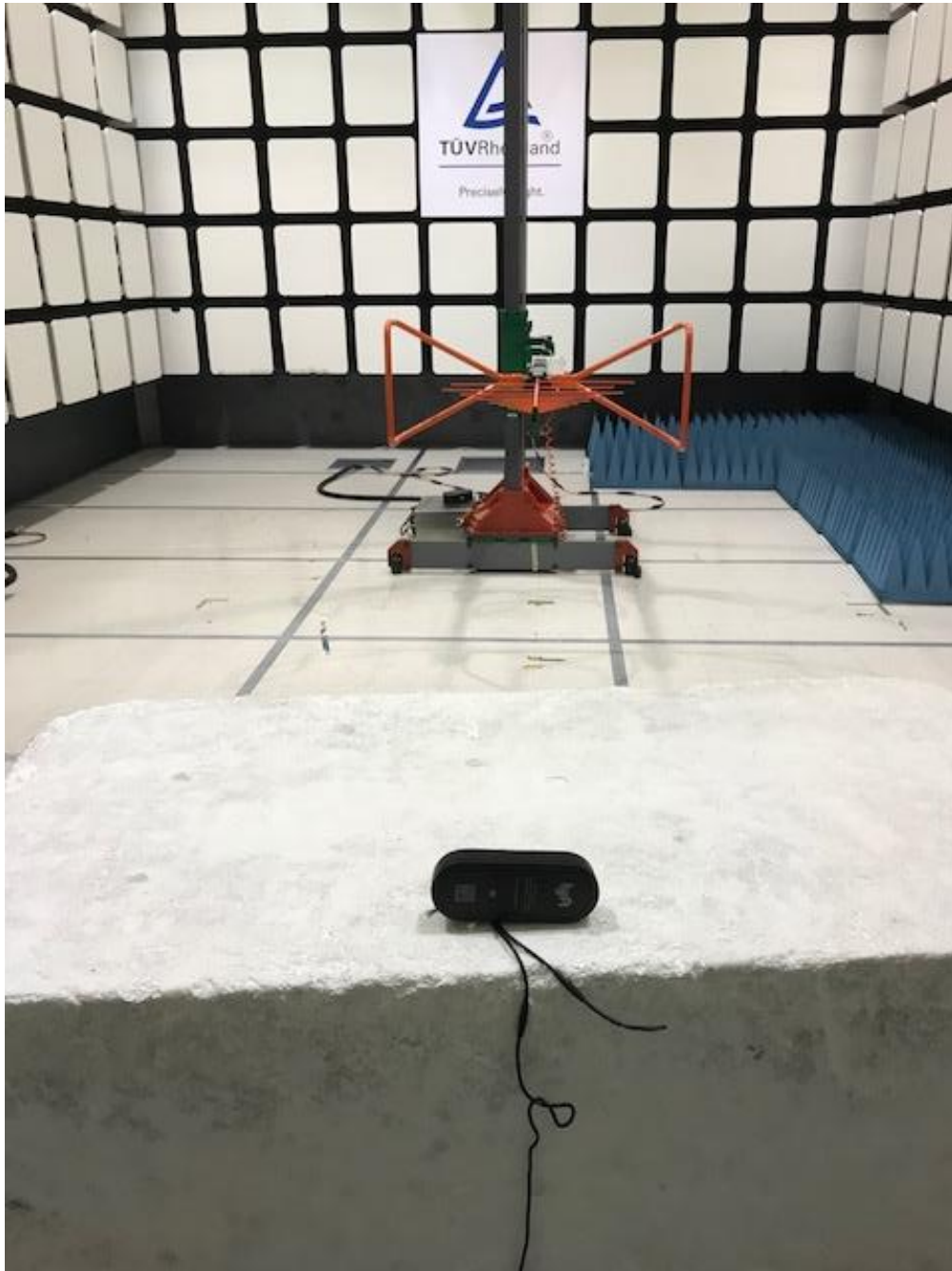
Figure 4 - Radiated Emissions Test Setup 30 - 1000 MHz - Back
