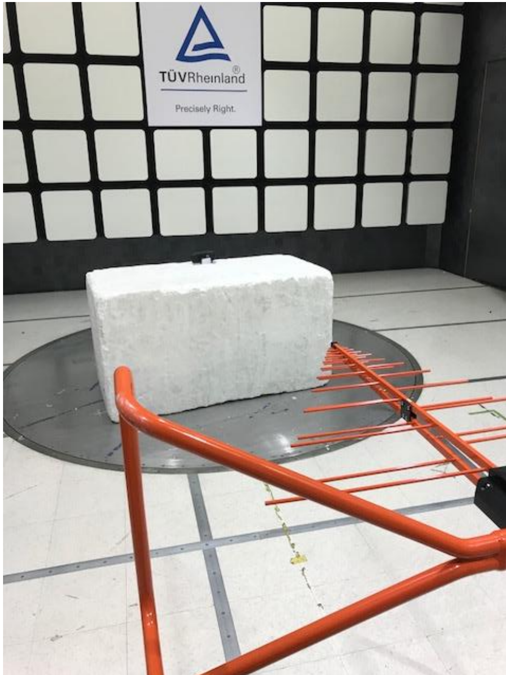
Figure 3 - Radiated Emissions Test Setup 30 - 1000 MHz - Front
