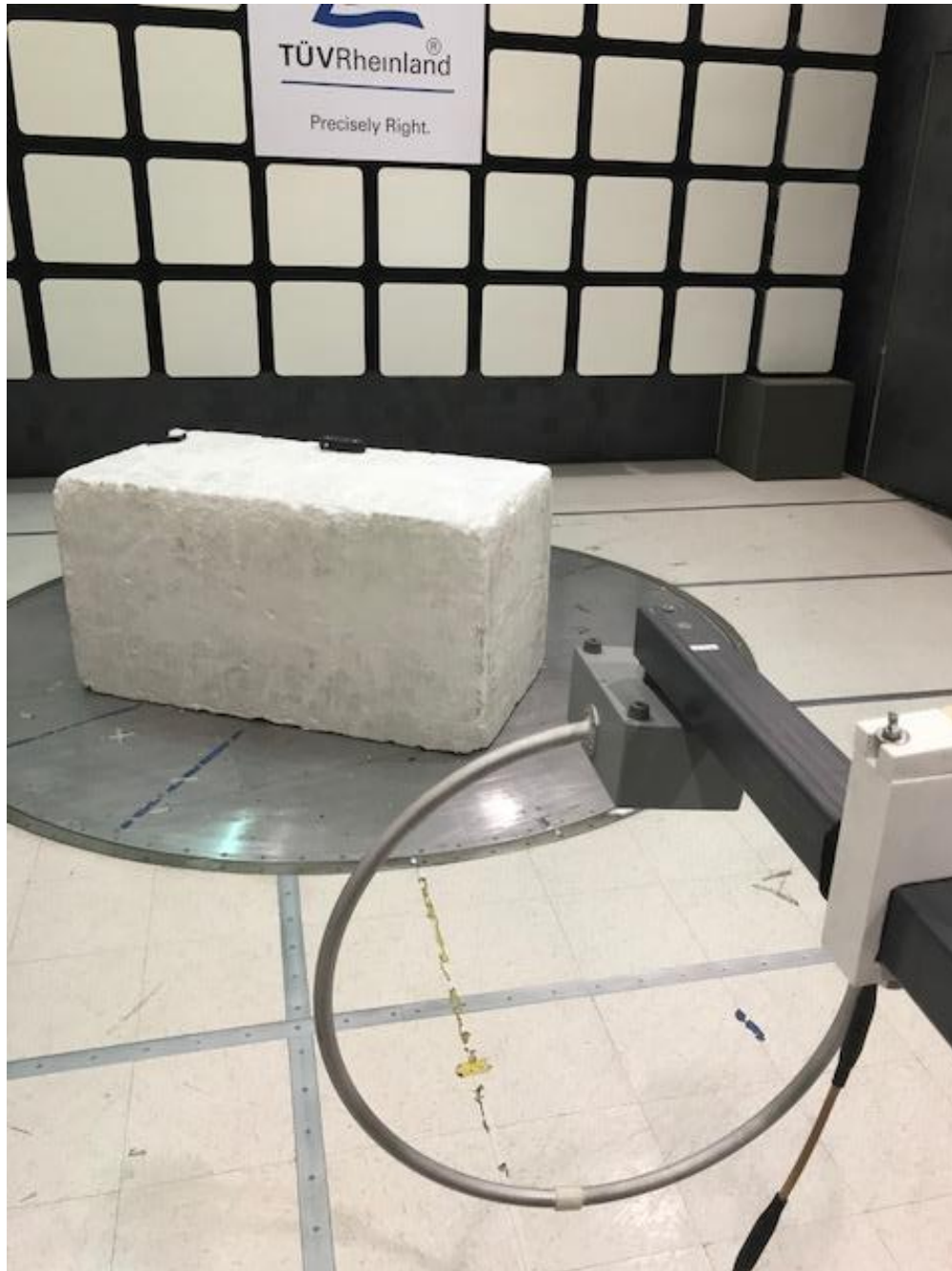
Figure 1 Radiated Emissions Test Setup 9 kHz- 30 MHz - Front
