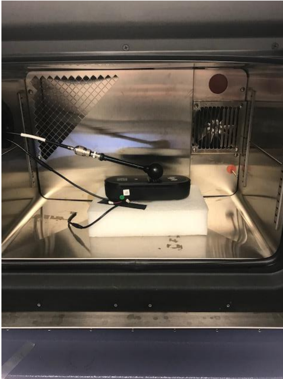
Figure 9 – Frequency Stability test setup
