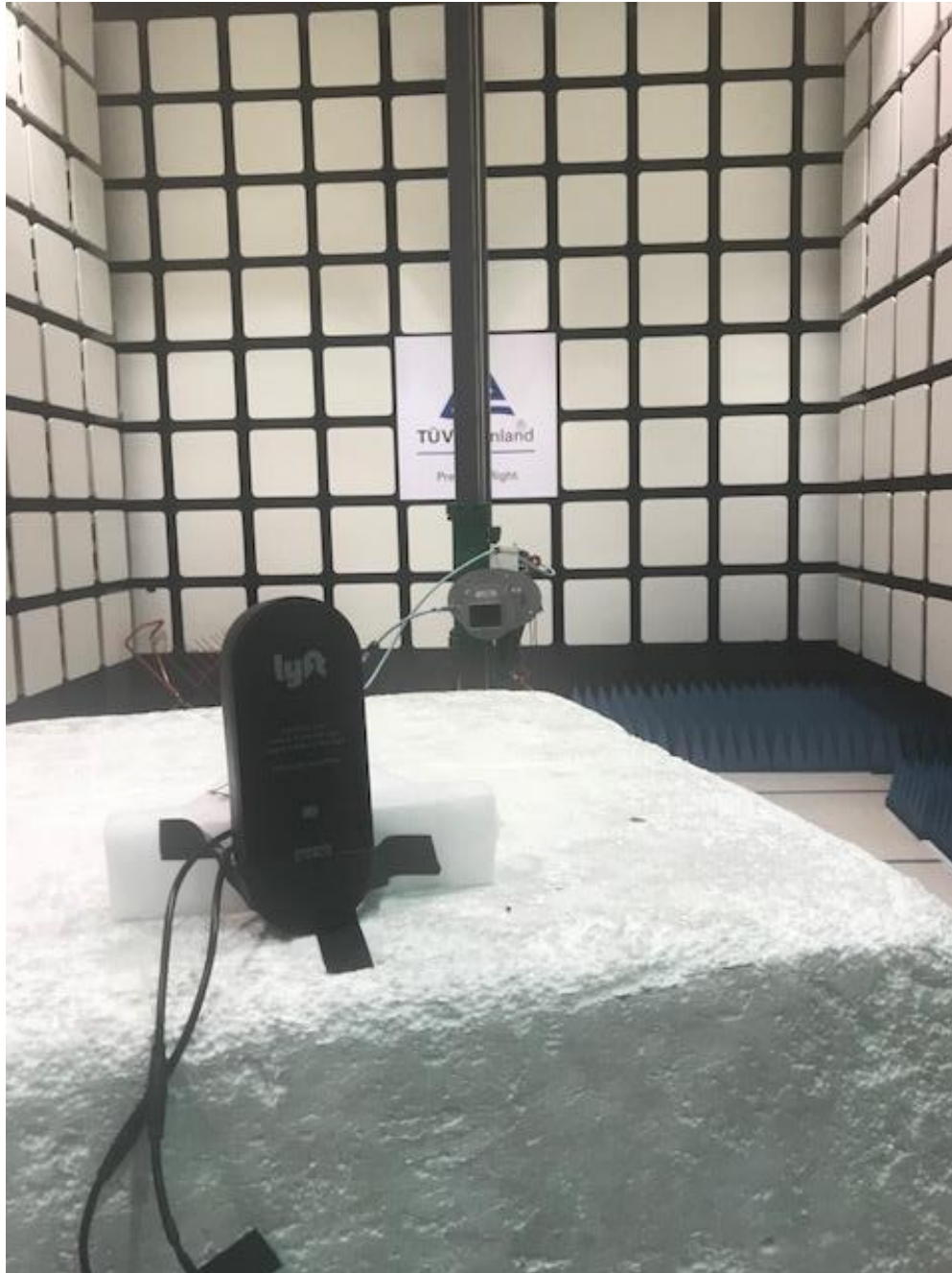
Figure 8 - Radiated Emissions Test Setup – 18-26 GHz Rear
