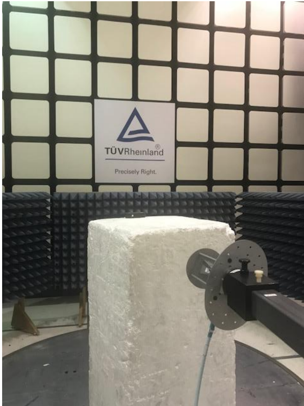
Figure 7 - Radiated Emissions Test Setup – 18-26 GHz Front
