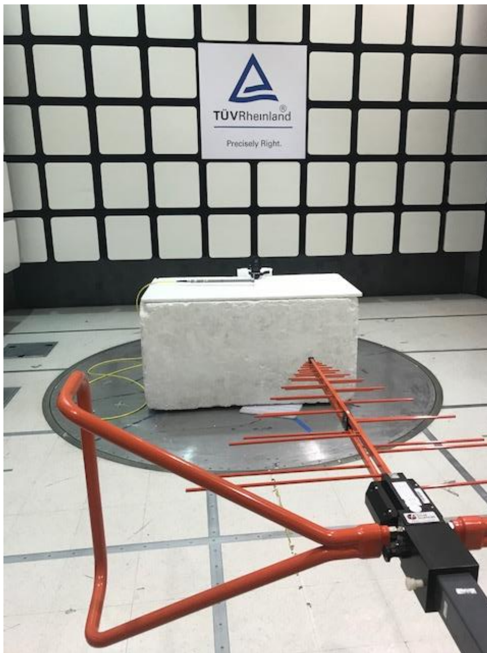
Figure 3 - Radiated Emissions Test Setup 30 - 1000 MHz - Front
