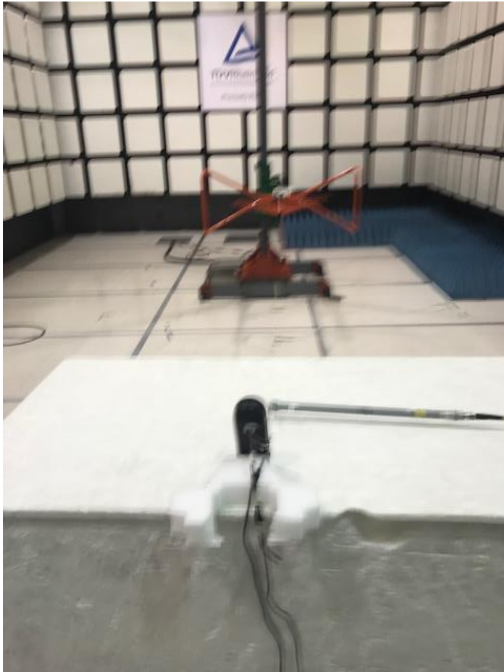
Figure 4 - Radiated Emissions Test Setup 30 - 1000 MHz - Back
