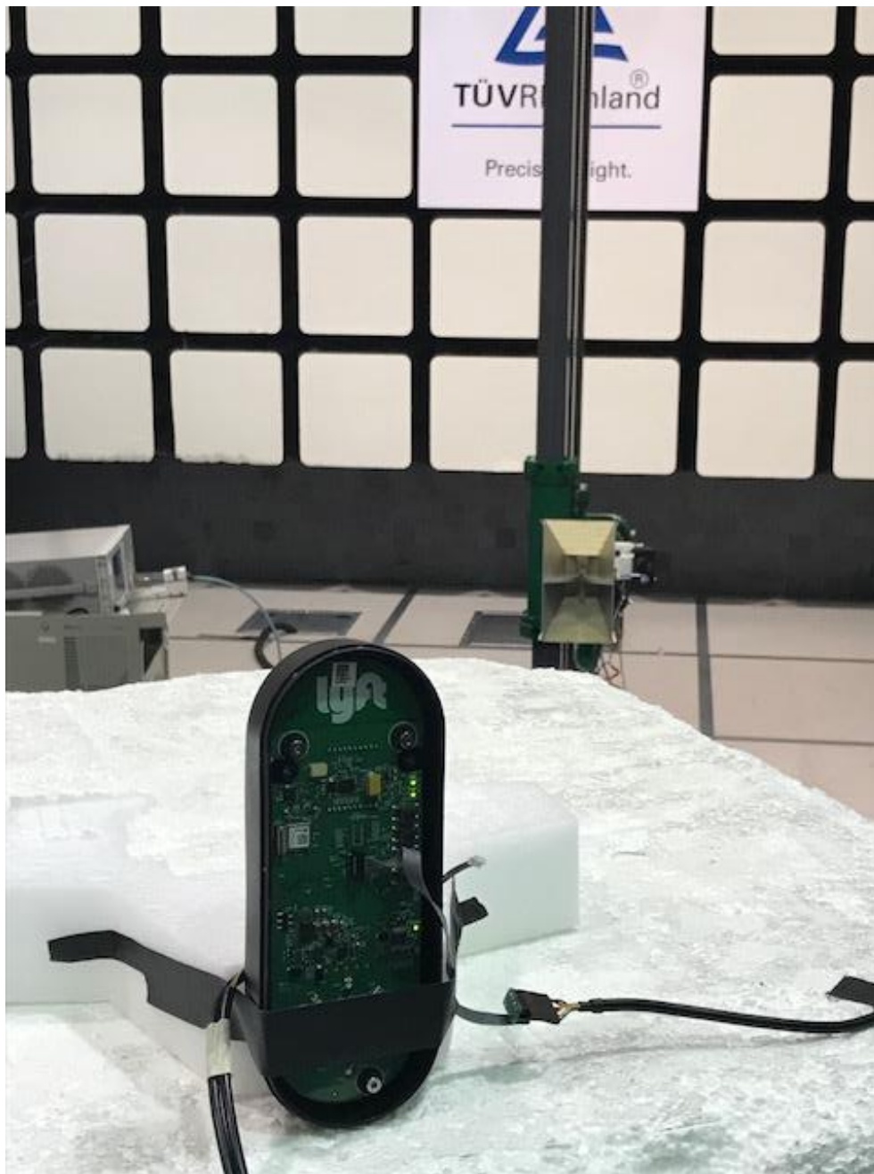
Figure 6 - Radiated Emissions Test Setup – 1-18 GHz Rear
