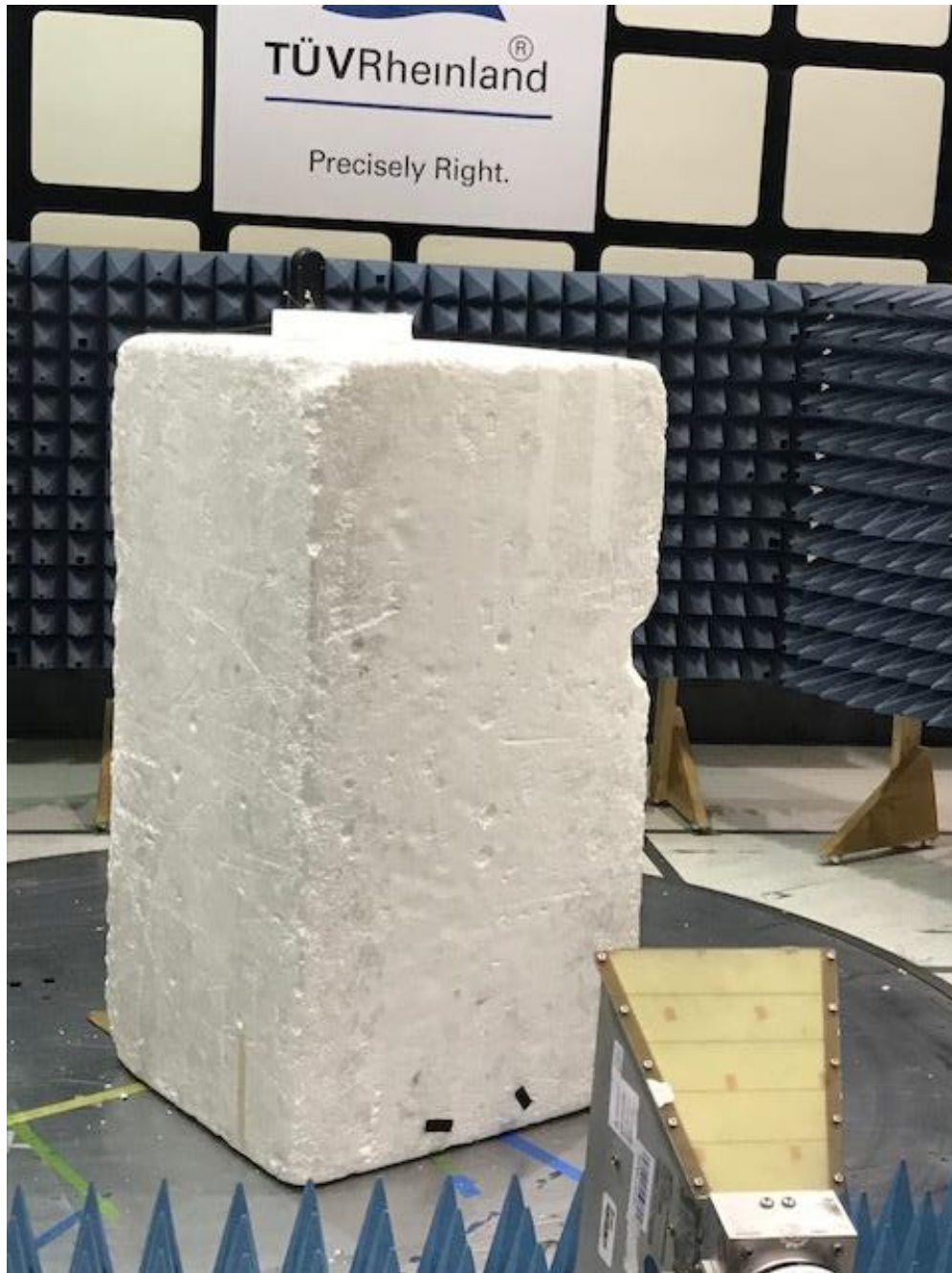
Figure 5 - Radiated Emissions Test Setup – 1-18 GHz Front
