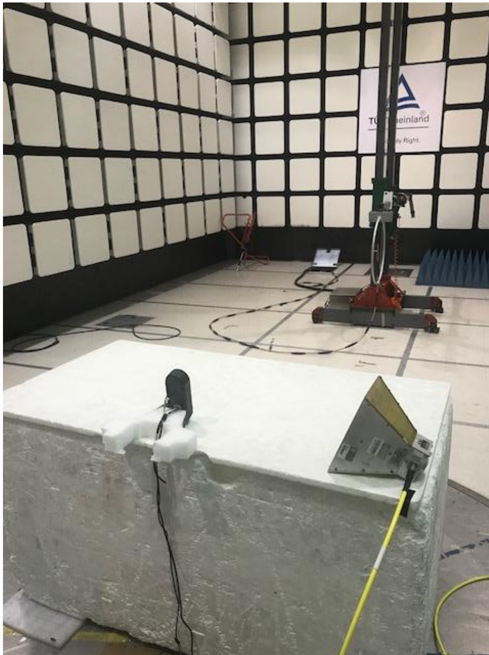
Figure 2 - Radiated Emissions Test Setup 9 kHz-30 MHz - Back
