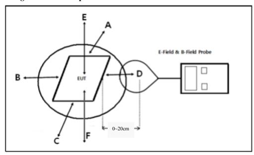
Note: The EHP-200AC Probe has a diameter of 9.2cm and a radius of 4.6cm.
