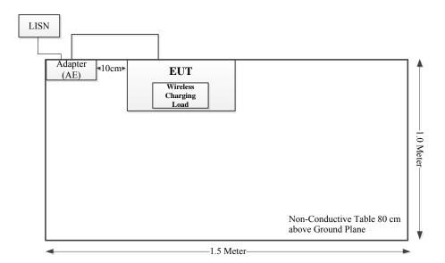
Radiated Emission Test M1:
