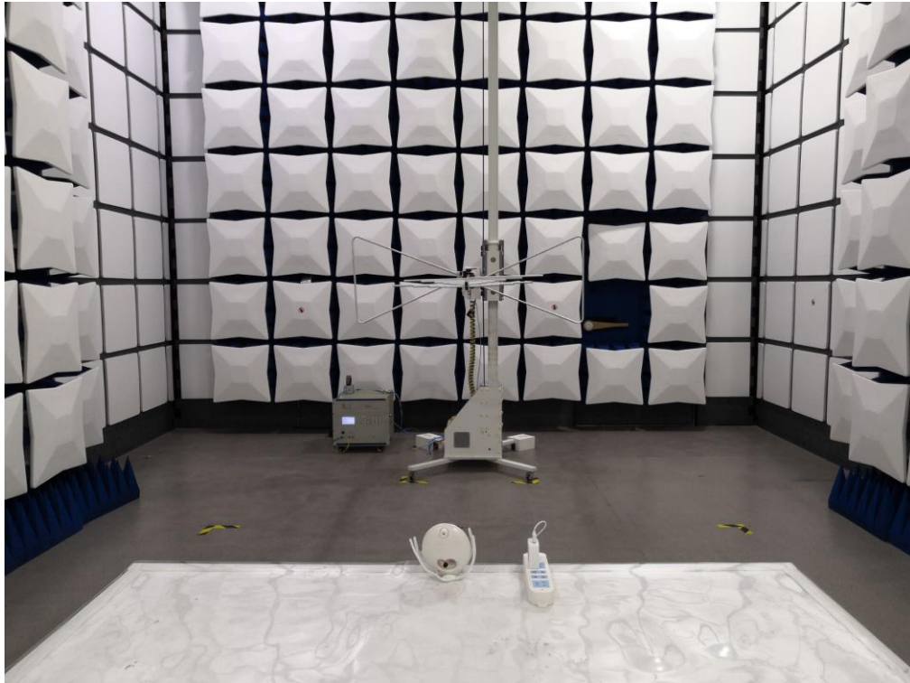
FCC RADIATED EMISSION TEST SETUP ABOVE 1GHZ
