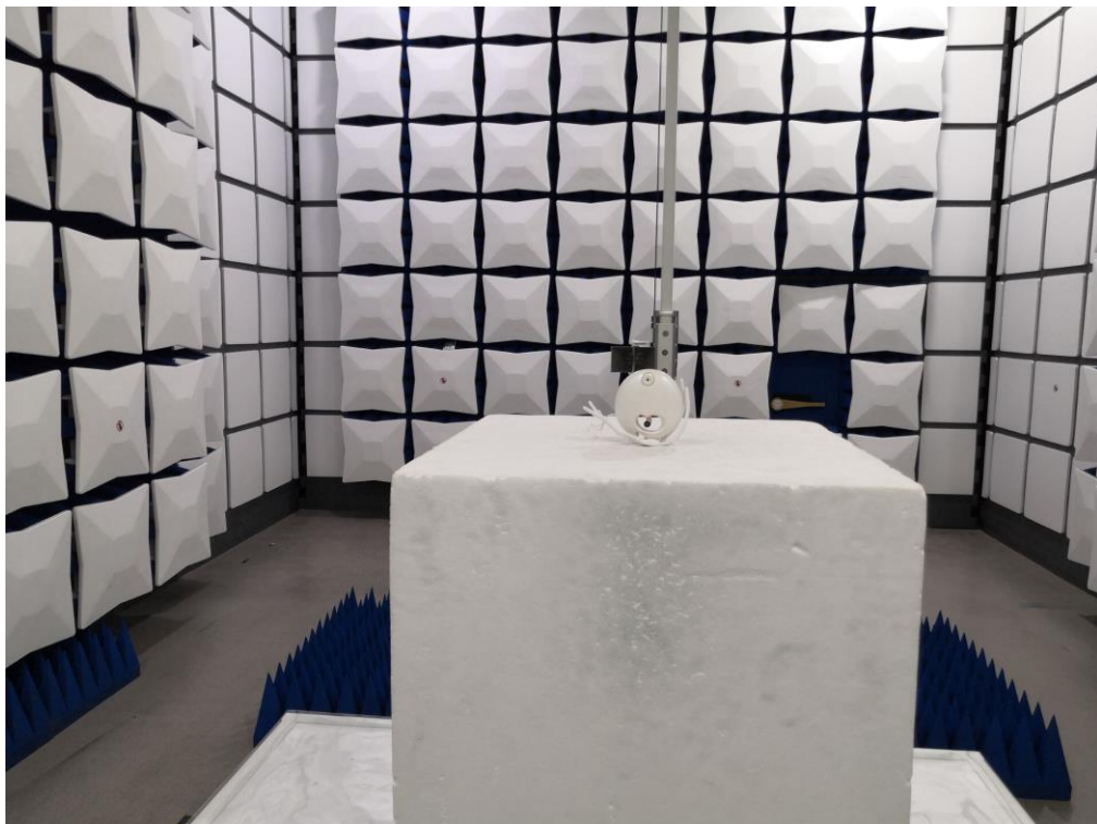
FCC RADIATED EMISSION TEST SETUP ABOVE 1GHZ
