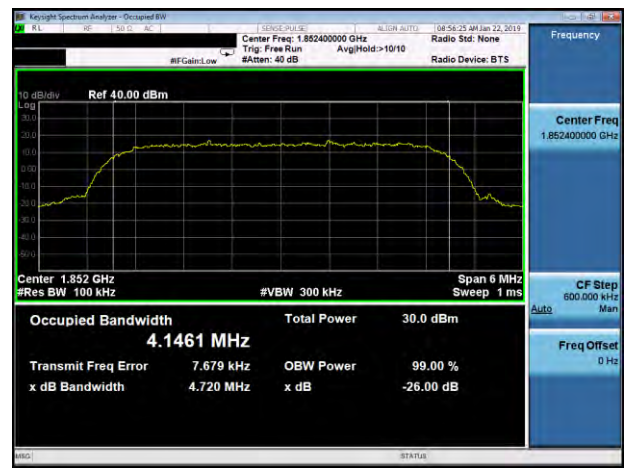
-26dB&99% Bandwidth plot on channel 9400
