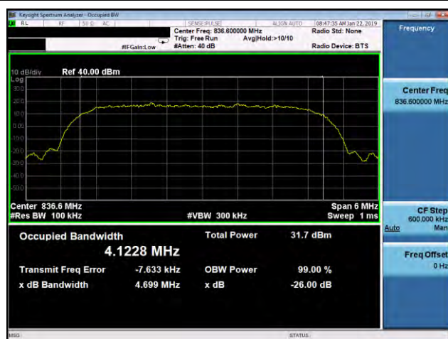
-26dB&99% Bandwidth plot on channel 4183
