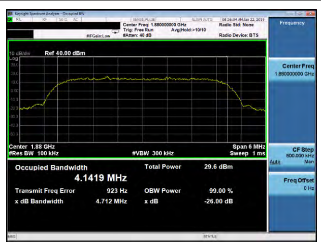
-26dB&99% Bandwidth plot on channel 9400
