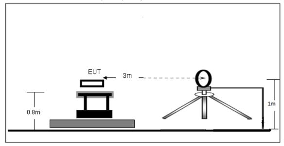
(B) Radiated Emission Test-Up Frequency 30MHz~1GHz
