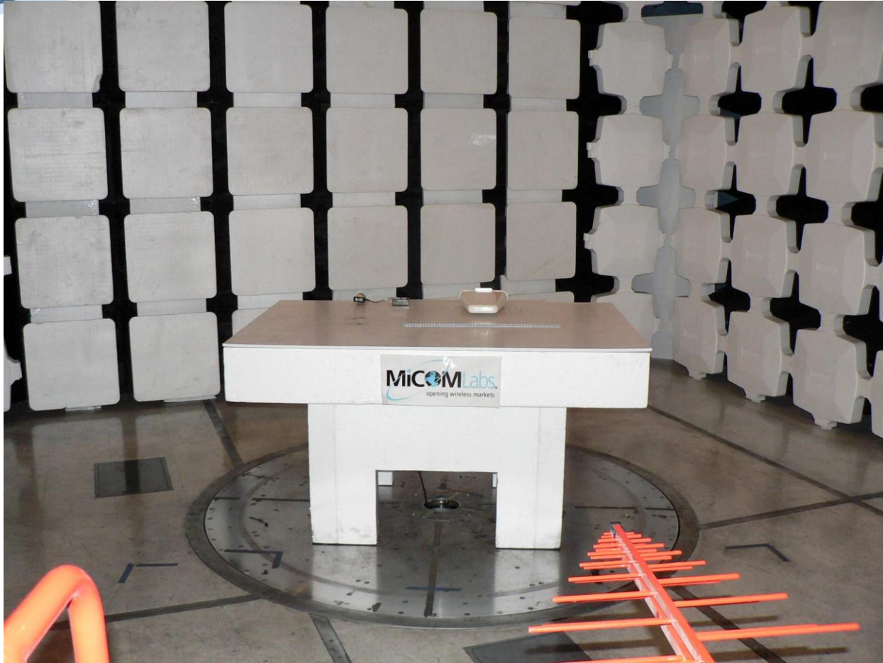
PULO01 TX Spurious 30-1000MHz Yagi Antenna
