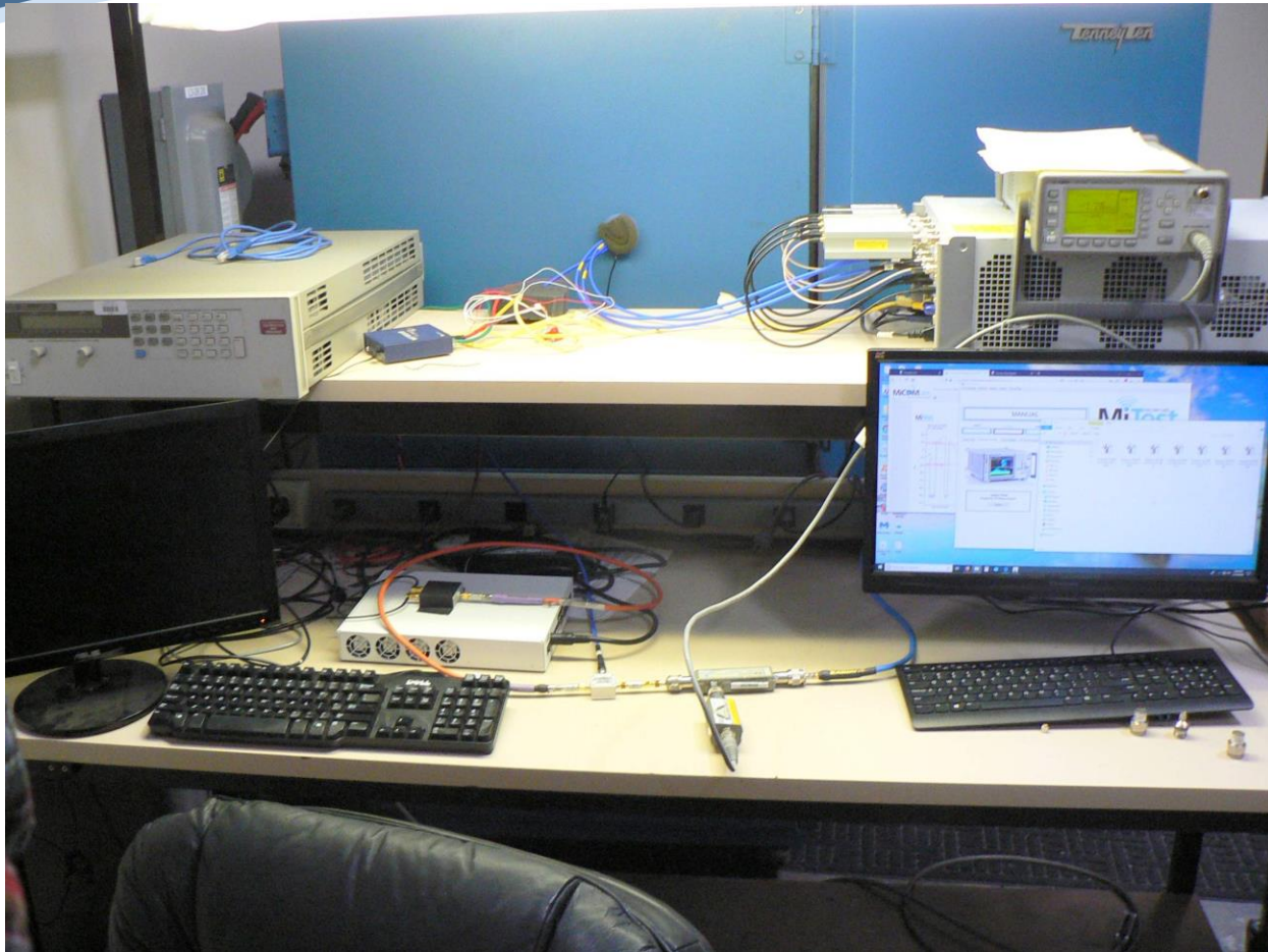
PULO01 RF Conducted Test Setup
