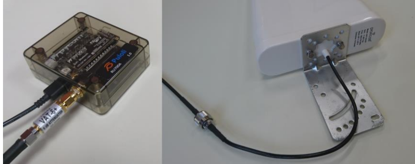
Figure 3. Yagi antenna with attenuator and SMA-male to N-male coaxial patch cable
