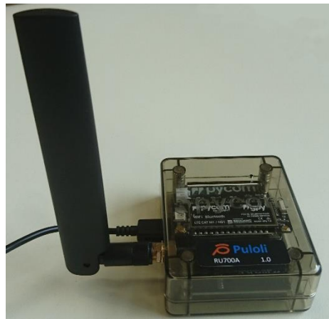
Figure 2. Indoor antenna configuration
