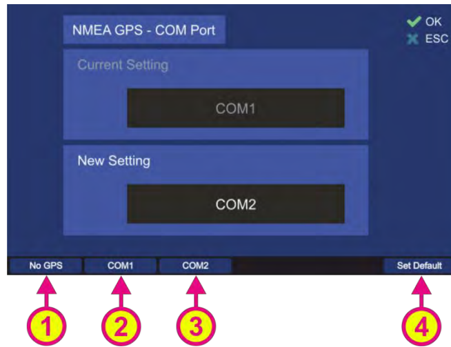
Figure 121. NMEA GPS communication port settings
