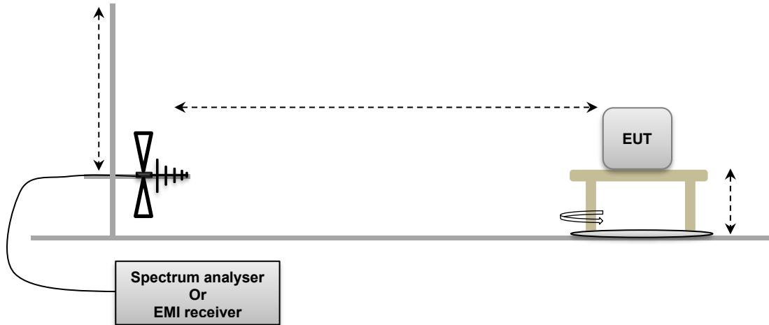
*Test setup of Radiated Emission*
