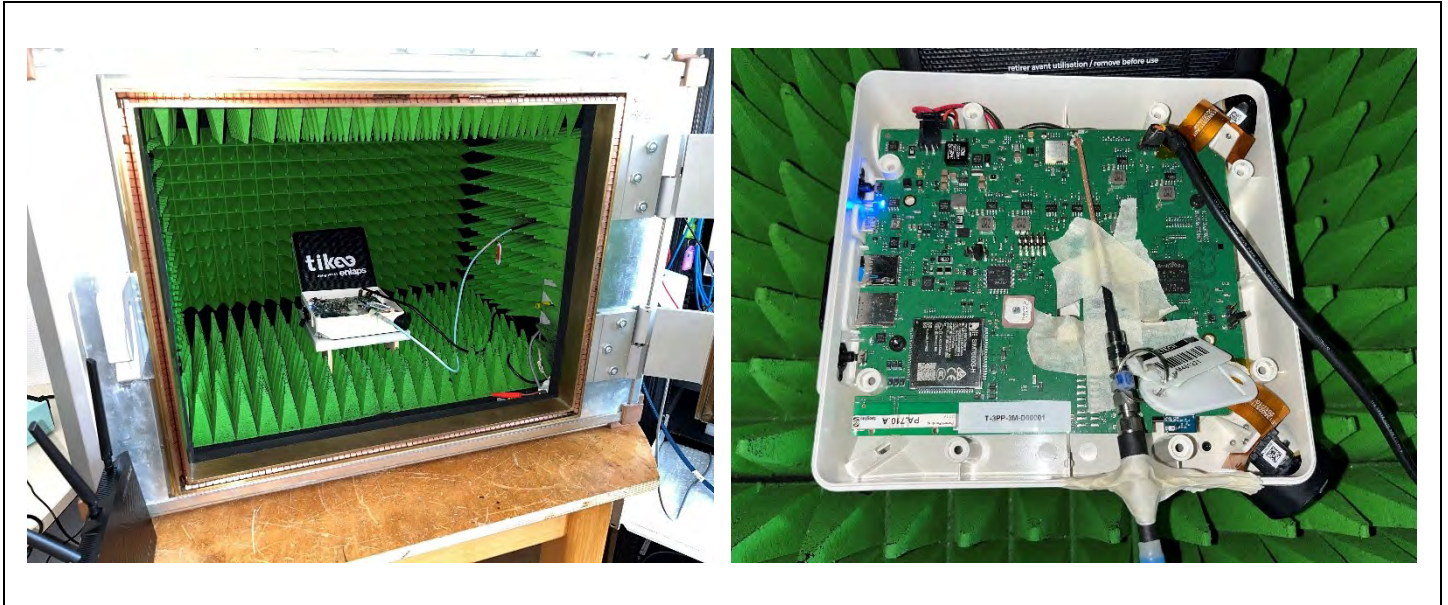
Photograph for Unwanted Emission into non-restricted frequency bands at the band edge
