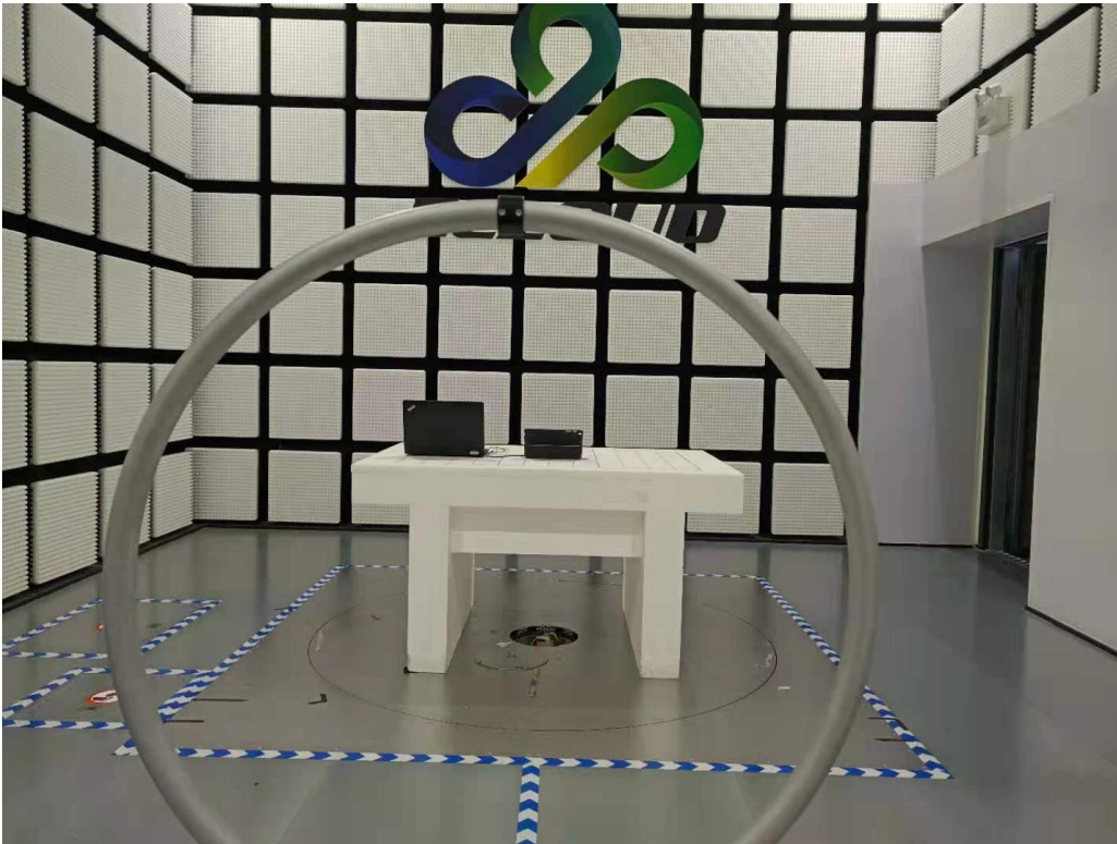
Fig. 1 Radiated emission setup photo(Below 30MHz)
