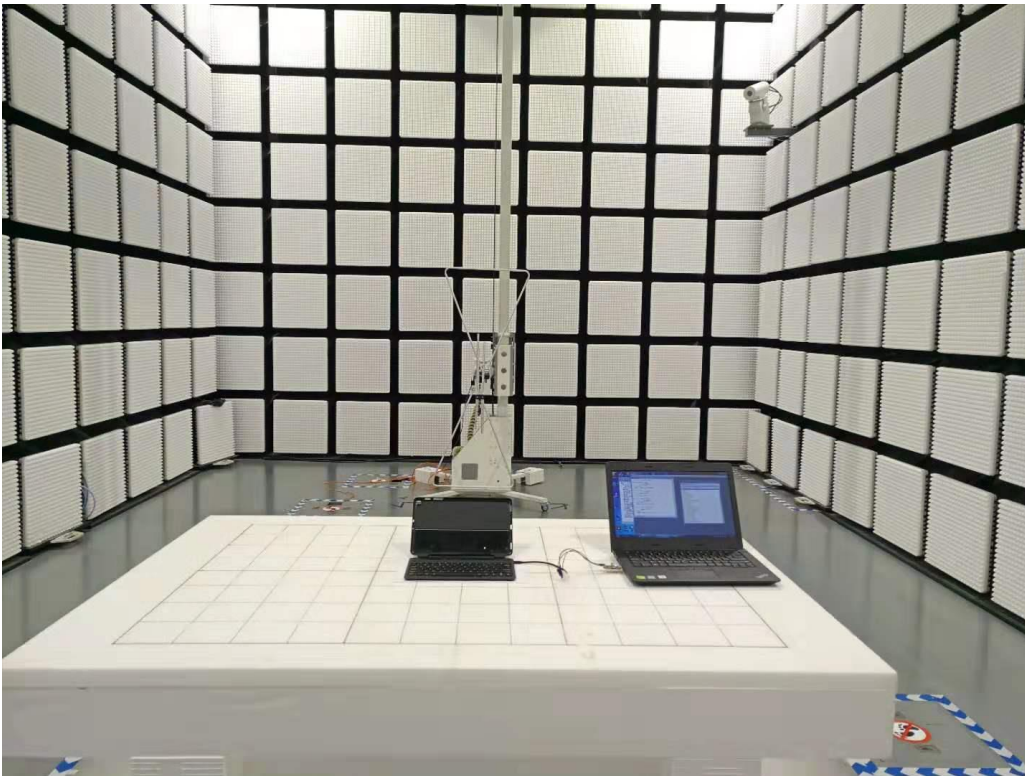
Fig. 2 Radiated emission setup photo(30MHz-1GHz)
