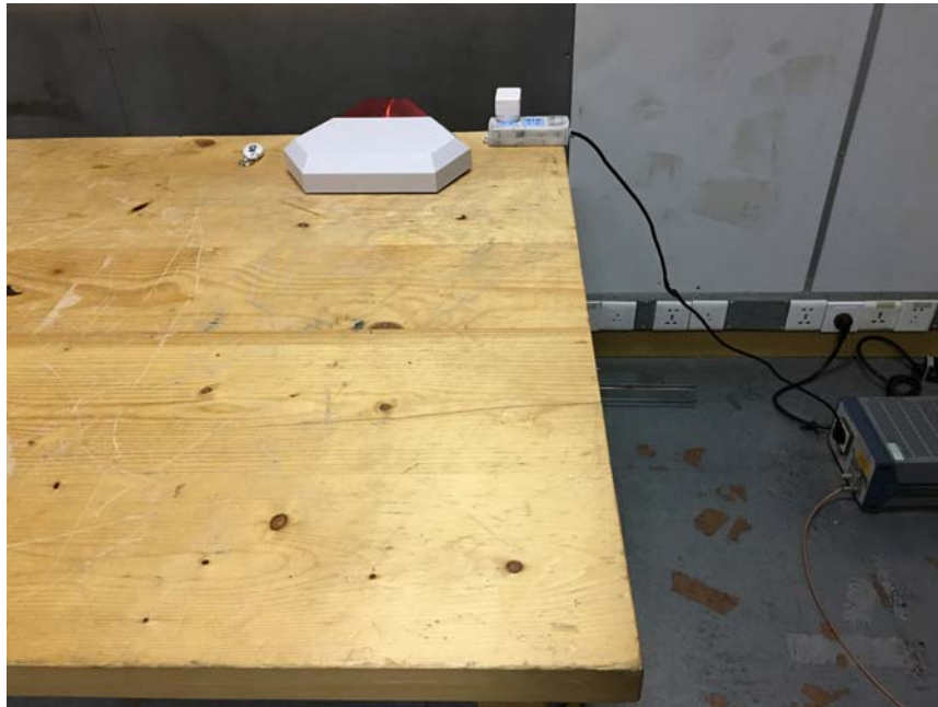
Photograph of set-up for conducted Emission
