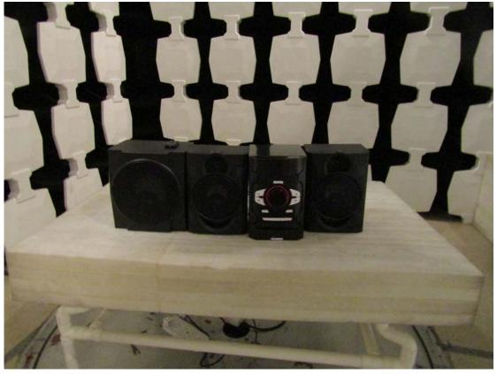
**Measurement of Conducted Emission Test Set Up**
