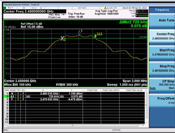
GFSK (BLE 1Mbps) HIGH CHANNEL
