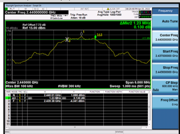
GFSK (BLE 2Mbps) MIDDLE CHANNEL
