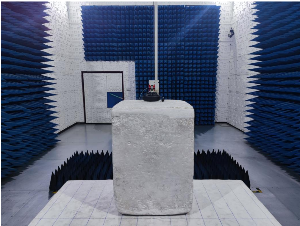
RADIATED EMISSION TEST SETUP ABOVE 1GHZ
