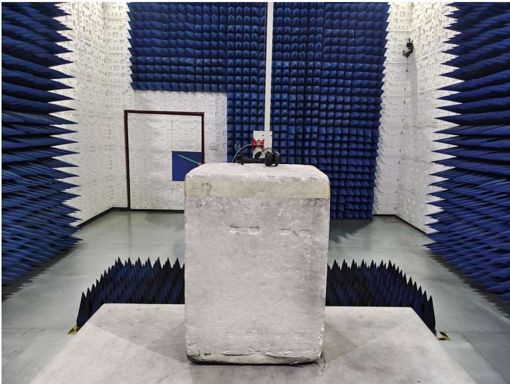
RADIATED EMISSION TEST SETUP ABOVE 1GHZ
