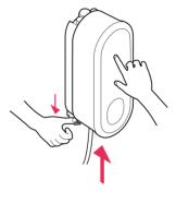
Keep a firm hold on the eBox while pulling down the locking bracket on the eClick. Now release the locking clip. As soon as the locking clip is pulled up, strongly press the eBox onto the eClick.
