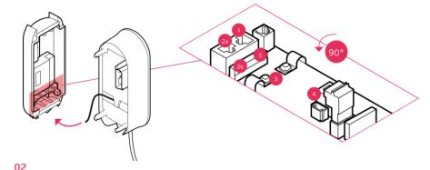
Connect the black ribbon data cable of the eBox to port 4 (Expansion terminal) at the bottom right of the eClick.
