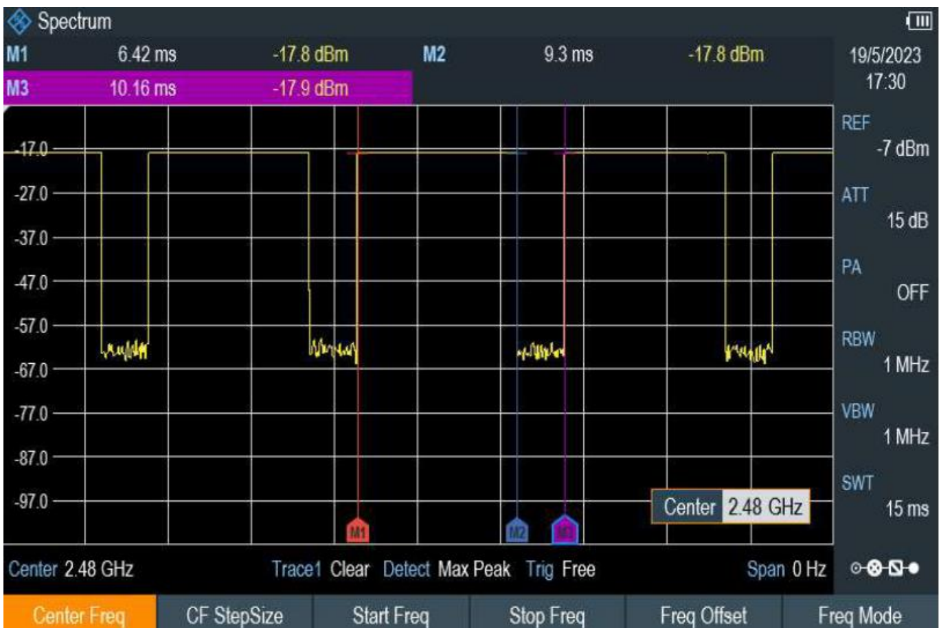
Time-domain plot for Bluetooth transmission signal
