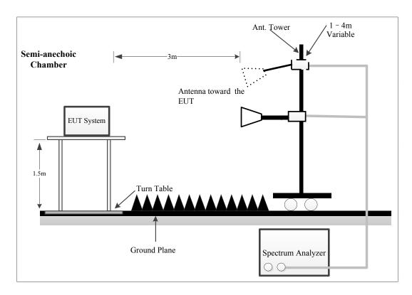
The radiated emissions were performed in the 3 meters distance, using the setup accordance with the ANSI C63.10-2013. The specification used was the FCC 15.209, FCC 15.247 limits & RSS-247, RSS-Gen limits.
