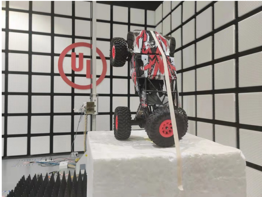
Radiated Disturbance Setup (Above 1 GHz – Z axis)
