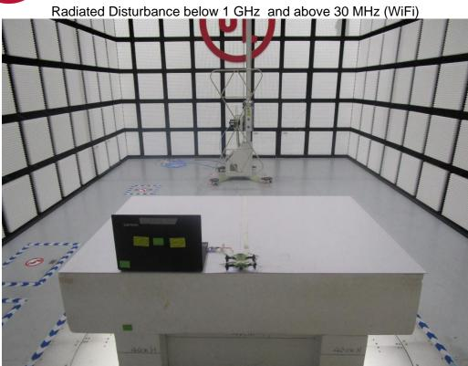
Radiated Disturbance below 1 GHz and above 30 MHz (2.4 GHz)
