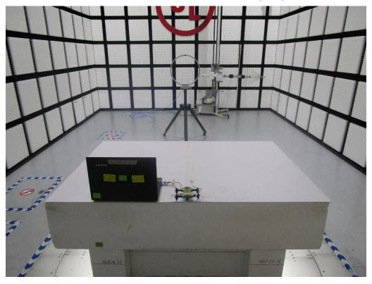
Radiated Disturbance below 30 MHz (2.4 GHz)
