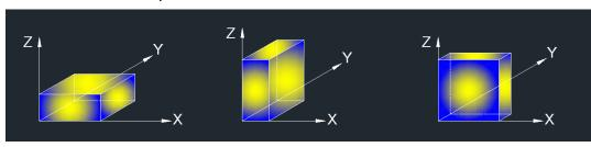
Note 1: For all radiated test, EUT in each of three orthogonal axis emissions had been tested, but only the worst case (X axis) data recorded in the report.
