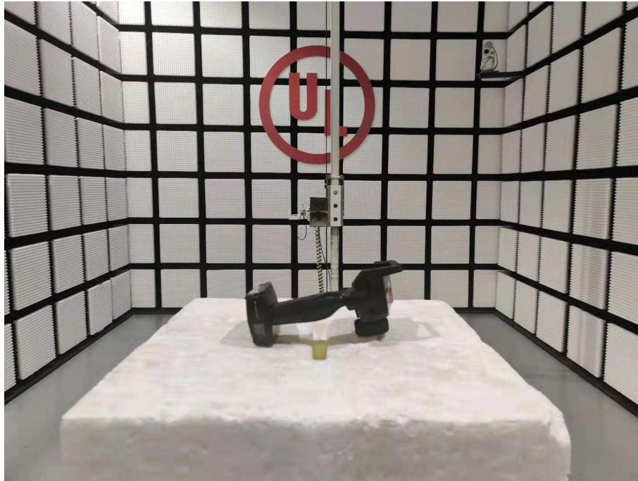
Radiated Disturbance Setup (Above 1 GHz – Y axis)
