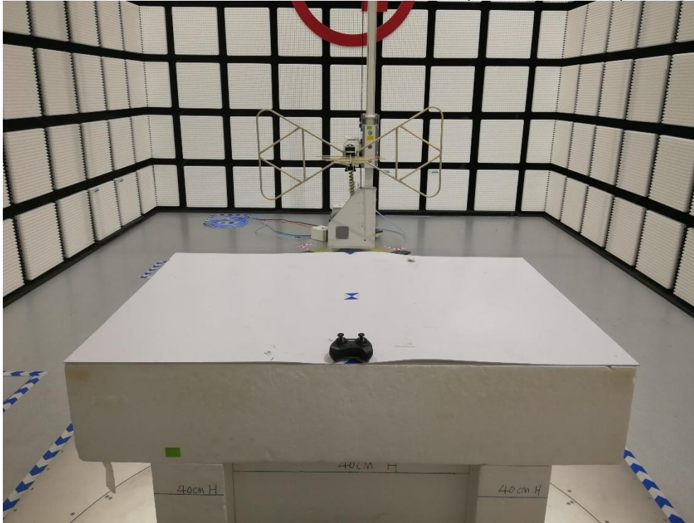
RADIATED RF MEASUREMENT SETUP (30MHz ~ 1 GHz)
