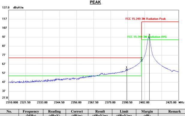
(MHz) (dBuV) (dB/m)(dBuV/m) (dBuV/m) (**dB**) 1 2390.000 27.35 32.94 60.29 74.00 -13.71 peak 2 2400.000 37.76 32.98 70.74 74.00 -3.26 peak 3 2405.220 63.30 33.02 96.32 114.00 -17.68 peak
